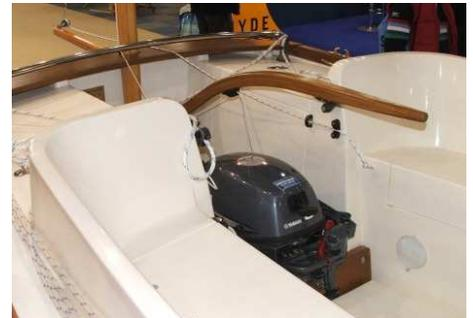
Some customers have fitted Mariner/Tohatsu engines & like them (though one customer fitted a Tohatsu & complained bitterly about fumes exiting the bypass partway up the leg & filling the cockpit). Some have increased from 8 to 9.9 (basically the same engine) so that they can specify electric start. I have never felt the urge to do this.
