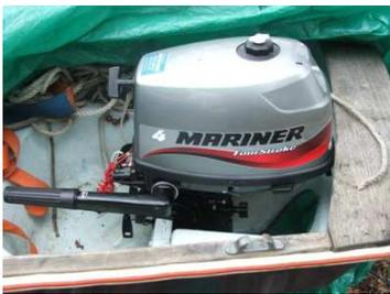
Some people do fit a 4hp but there are down-sides. I wouldn't be doing that myself. That may require trimming away a bit of the transom board to allow the engine to turn & some introduction of primary wedges between outboard pad & hull or secondary wedges (see below) on the back of the outboard pad. Both will change the angle of
