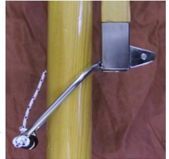
Its function is to stop the lower end of the yard escaping off the mast. In combination, the length & angle of the gaff jaws & the length of the parrel bead string need to be enough to allow the yard to drop down to the horizontal & maybe even a bit beyond.
