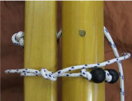
The third string of 4 beads is an optional one with pros & cons, requiring a Skipper's decision. It is tied on round yard & mast just below the halyard attachment point. (Put it through a loop of your sail lace marline hitch to keep it located on the yard. There is no lacing in the picture!)
