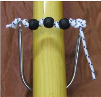
The 3 bead string goes through the gaff jaws. It is tied eccentrically with one long tail & one short one. Tie the short tail permanently onto the Port tang of the jaw. Tuck the loose end down the polythene tube protector (if you have them). In use, thread the free end through the Starboard tang & tie off with two half hitches or any other exotic bend that takes your fancy.
