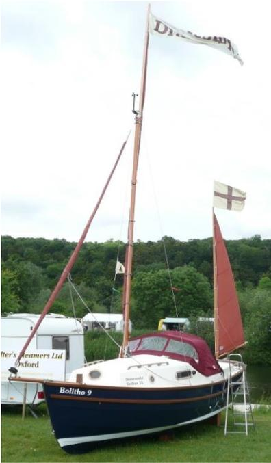
I am a great fan of The Harbour Furl, by which I mean rolling the mainsail tightly around its own leech up to the mast & securing it with a couple of ties as in this picture.
