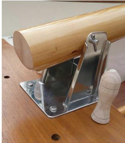
On the cabin boats, the mainmast is stepped in a tabernacle, which is basically a pivot that allows the mast to hinge.
